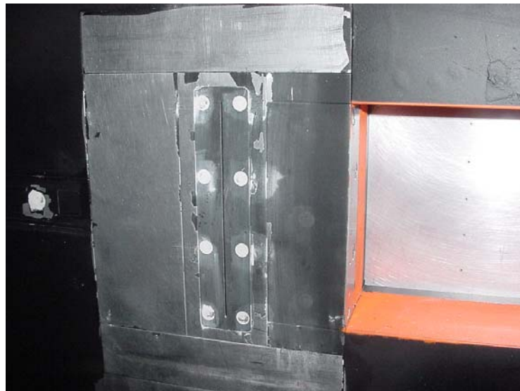
Figure 4: Microjet arrays located upstream of the HIFEX weapons bay
