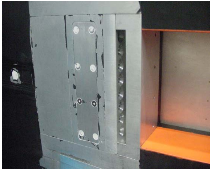
Figure 1: 10%-Scale HIFEX weapons bay model installed in Boeing Polysonic Wind Tunnel
